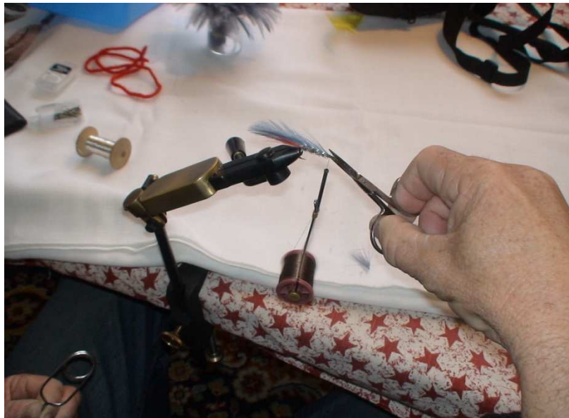
Photo 26: trim off excess - note angle.
